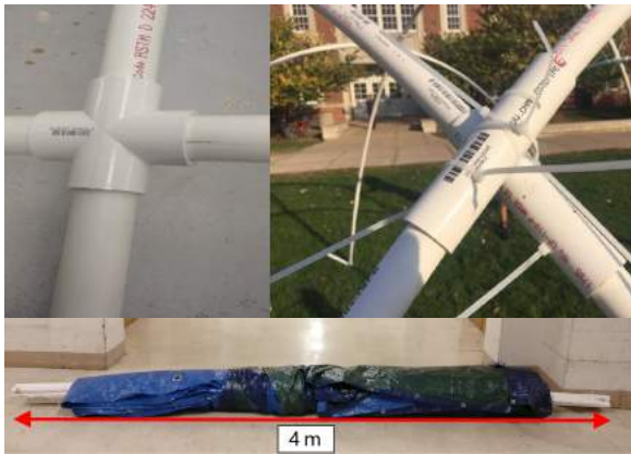
Original and revised joint designs
