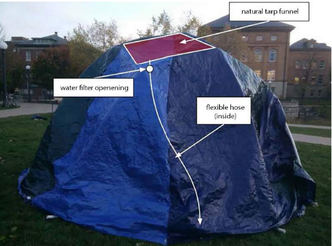
Final prototype with water collection schematic
